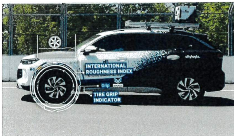
The Tire Grip Indicator, mounted on the survey vehicle, measures International Roughness Index during the core survey pass
