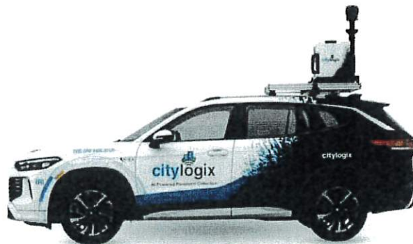
Citylogix pavement data collection vehicle equipped with LiDAR, 360° cameras, and GPS/IMU systems
